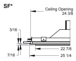
\* For SF spplications, a separate trim frame ships with a LT diffuser
