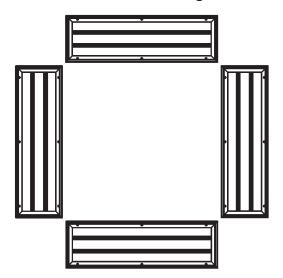
The plenum elbows allow for continuous plenum configurations as shown. Two elbows reduce the number of inlets from four to two. If a single inlet is required, four elbows would be utilized.
