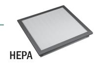
High Efficiency Particulate Air Filter to accommodate the TENSOR  $^{\mathsf{TM}}$  (or Subplenum model if baffle is removed) and Vector  $^{^{\otimes}}$ -H HEPA model for critical environments. Designed with the Dimple Pleat media pack which does not require glue, strings or strips of media to hold adjacent folds of media apart and gives the media pack its shape and strength. Such materials are potential sources of particle generation.
